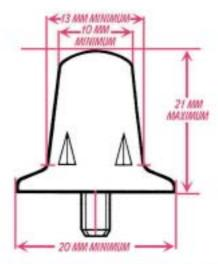
THE MAXIMUM AND MINIMUM DIMENSIONS OF A STUD ARE SHOWN HERE.
